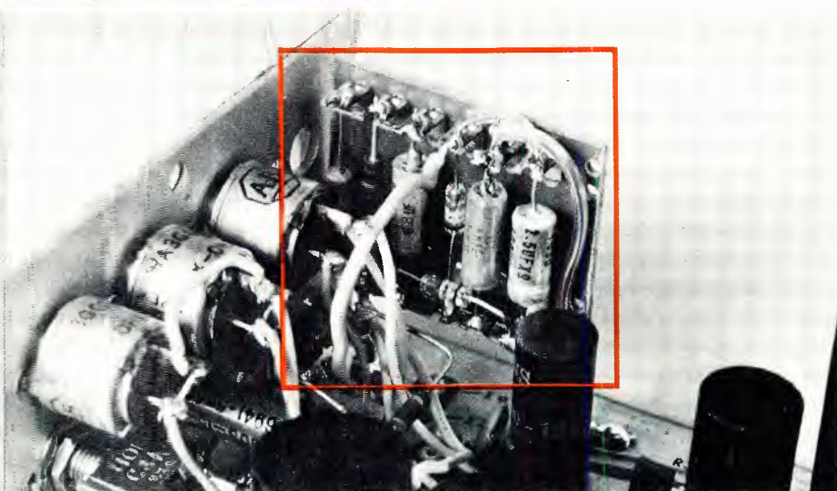
Fig. 2 Blocked off area shows positioning of the PC board for enhancer modification.
